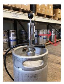
4) Press the nozzle on the tap with your thumb to allow the mead to flow out. To minimize foam, pour down the side of the glass and open the nozzle all the way, not half-way. Let the built-in pressure of the keg push the first couple drinks out; do not used the pump immediately. Once the initial pressure has subsided, pump the tap while the nozzle is open to push the mead into your glass. Enjoy!
