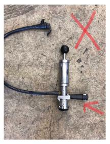
2) Align the coupler lugs with the corresponding openings in the tap and insert.
